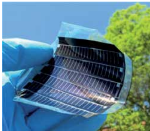
Figure 15. CdTe solar cells on colorless PI substrate (Source: Empa)
