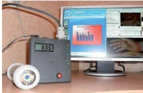
Figure 33. OEC components and probe express diagnostics of skin diseases (from left to right - probe measurement unit, PC). 1 - LED matrix, 2 - photodetector, 3 - protective optically transparent element, 4 - BO, 5 - enclosure.
