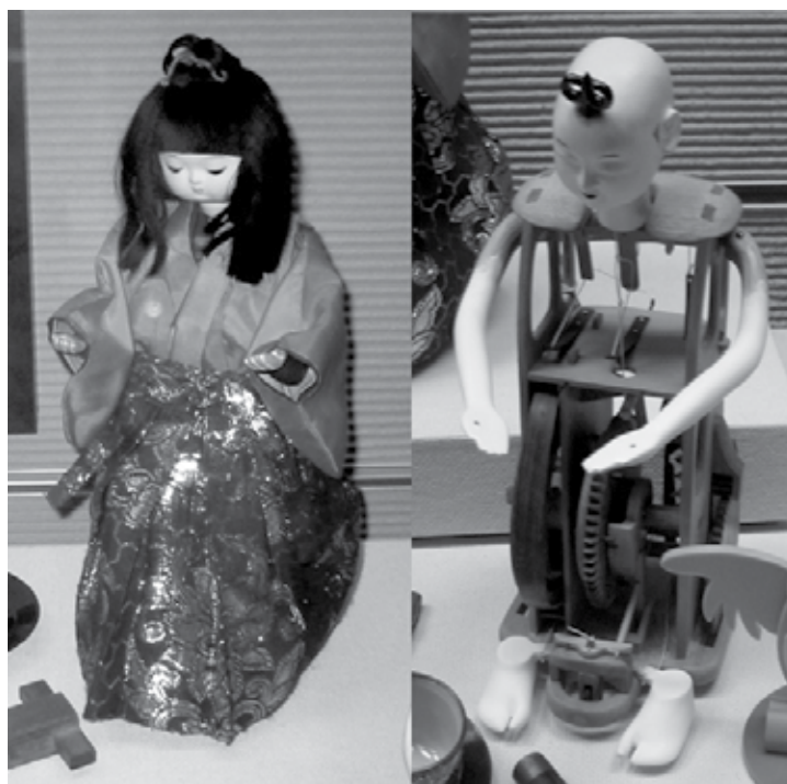
Figure 1. Karakuri ningyō (Japanese mechanized doll). This is a tea serving mechanized robot. The karakuri ningyō serves a cup of tea, and its sequence is roughly as follows: 1) When a cup of tea is placed on the hands, they start to move toward a guest by moving its feet like walking. 2) It moves, setting distance, and bows its head. 3) When a cup of tea is taken from the hands, it stops and waits for a next action. 4) It turns around and returns to the starting position (host's place) when an empty cup is placed on the hands. It works by springs. Only the examination of each mechanical gear would not help to understand the entire behavior of the doll. Picture is taken from Wikimedia Commons [3] and converted to gray scale
