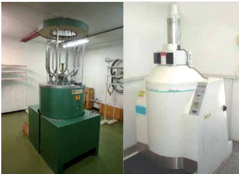
Figure 2. Types of gamma irradiators used in pest control trials or for disinfestation of commodities at the Center for Nuclear Energy in Agriculture (CENA, São Paulo, Brazil): (left) large-scale panoramic Gammabeam-650 irradiator; (right) self-contained Gammacell-220 irradiator.
