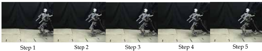
Fig. 13. Humanoid robot performs biped walking applying current parameters value: h=568 [mm], s=75 [mm] and d=0.8 , time per step 2.5 sec.
