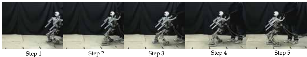
Fig. 12. Humanoid robot performs biped walking applying the best parameters value from simulation results: h=518 [mm], s=200 [mm] and d=0.7 , time per step 4.5 sec.
