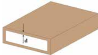
Figure 11. The cross section of a glass plate with a marked depth d of doped region.
