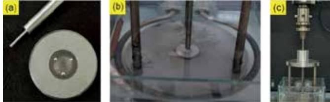
Figure 11. Images of biaxial flexural device: (a) loading piston and three-ball support; (b) disc specimen positioned in the flexural device and immersed in artificial saliva with heating element; (c) general view of the biaxial flexural loading device [5]
