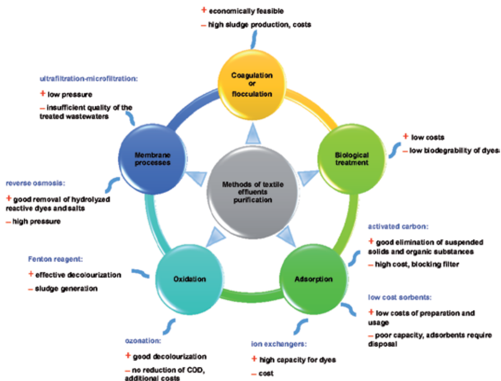
Figure 3. Advantages and disadvantages of the current methods of dye removal from industrial effluents
