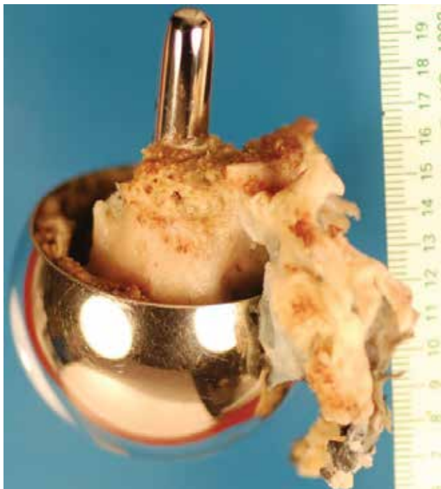
Figure 4. Retrieved head with extensive resorption of head osteolysis and growth of a pseudo-tumour
