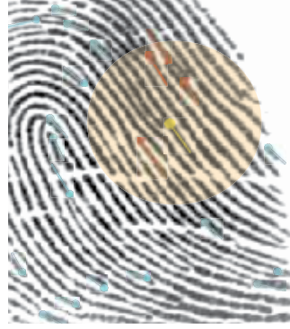
Fig. 12. The \delta -neighbourhood ( \delta = 4 ) for a given minutia (ignoring false crease minutiae).
