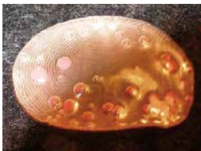
Fig. 2. Dummy fingerprint made by polymer.
