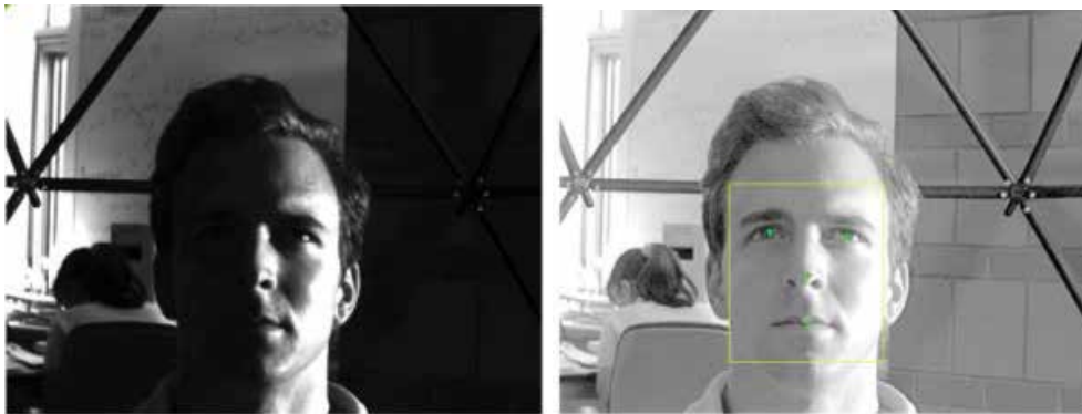
(a) Without preprocessing, face detector does not work (b) With preprocessing, face detector works well
