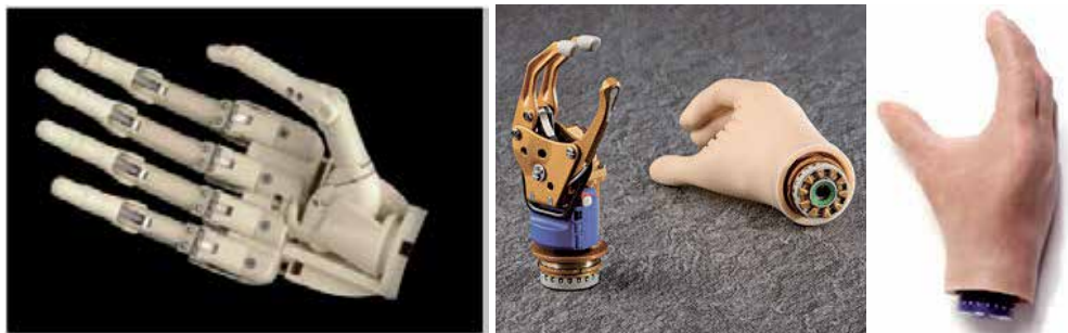
Fig. 1. Commercial prosthetic hands: a) Touch Bionics's i-Limb Hand, b) Otto Bock's SensorHand Speed, c) Motion Control Hand
