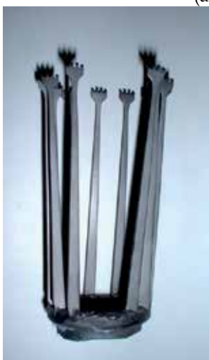
(b) Brain spatula just after precision casting
