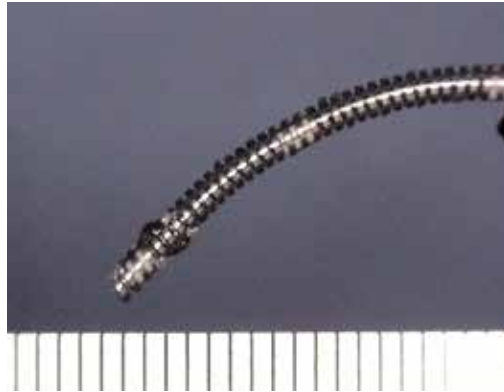
Fig. 5. Active bending catheter fabricated using electrodeposition (external diameter, 1.6 mm)
