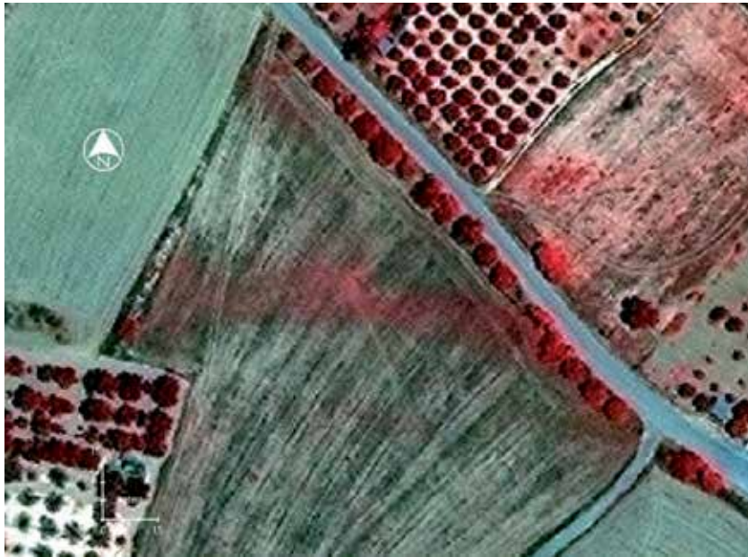
Figure 27. Detection of leakage problem using high resolution satellite data (Agapiou et al. 2014)
