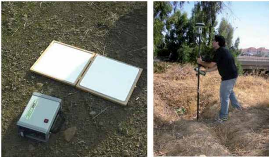
Figure 8. a) (left): The GER 1500 spectroradiometer used for the collection of ground measurements and b) (right): the GNSS used for mapping the pipeline
