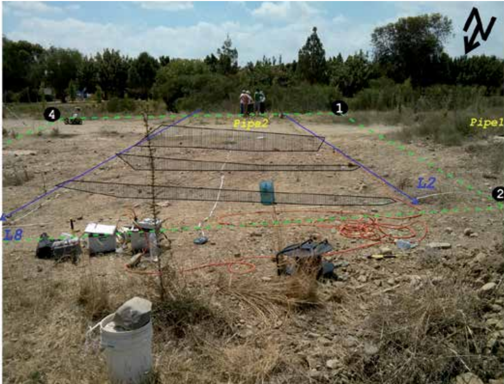
Figure 8. Outline of the footprint of water flow on the ground surface based on the results of the ERT monitoring experiment.
