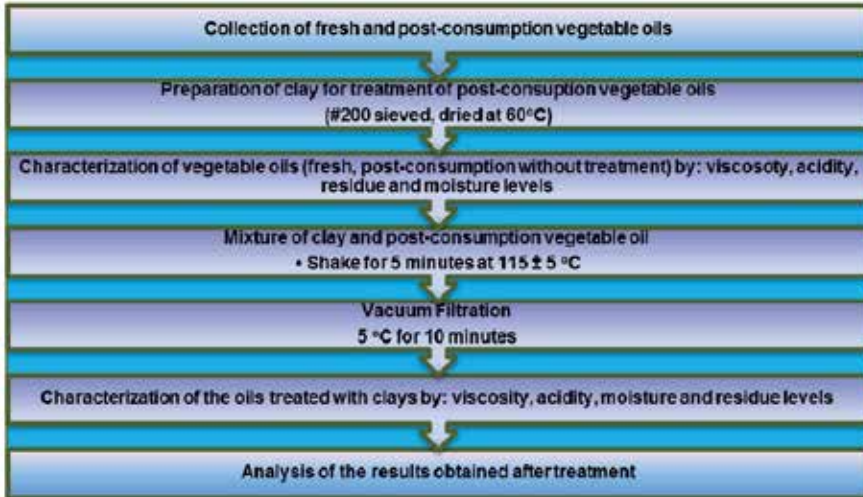
Figure 6. Steps in the treatment of post-consumer vegetable oils process.
