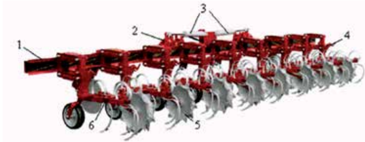
1 – frame; 2 – hanging device; 3 – hydraulic cylinders; 4 – regulation device for loosening depth; 5 – protective disc; 6 – section of ploughshares [27].
