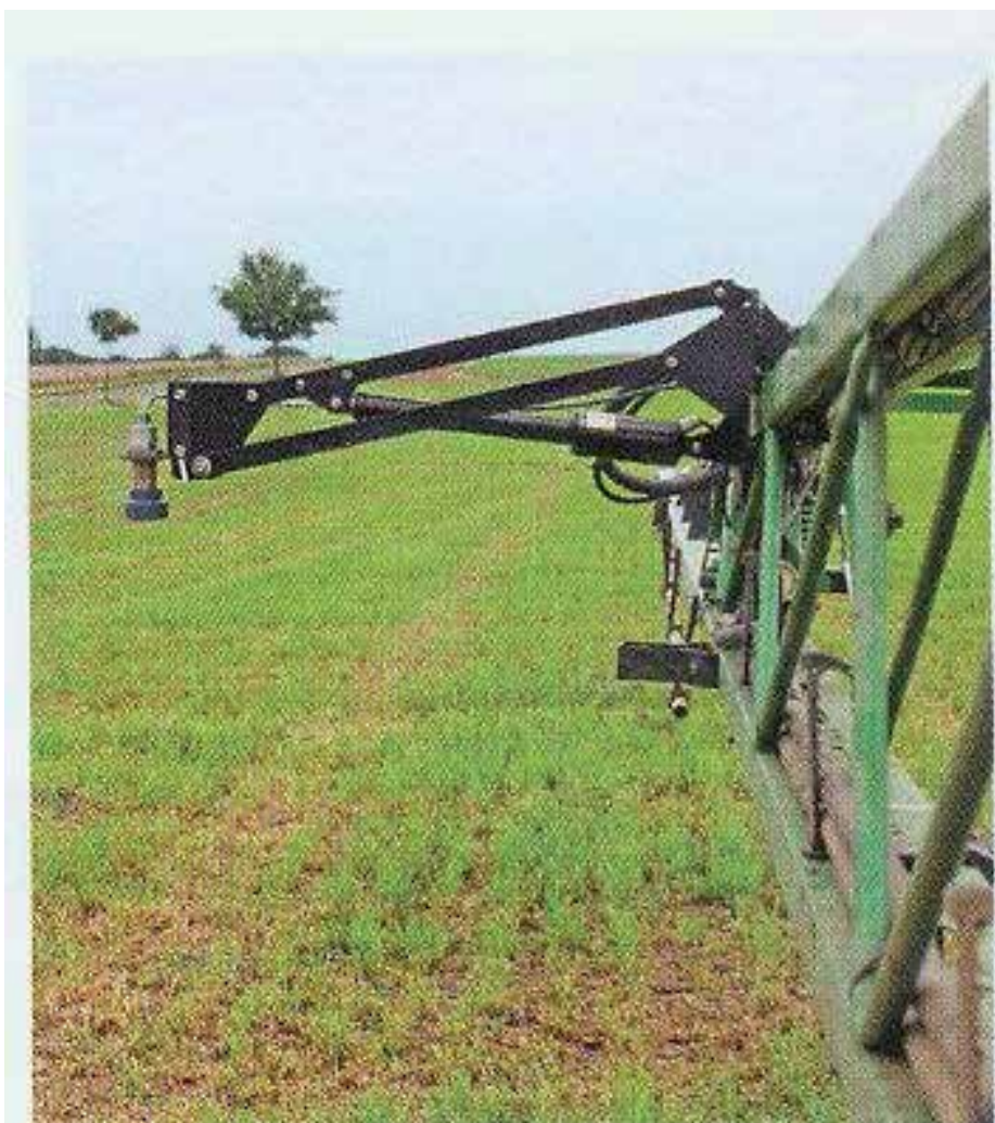
Figure 17. Ultrasound sensor P3 is attached to a field sprayer's beam for precise plant protection [24].
