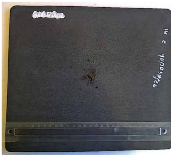
Figure 1. A macro etched cross-section from a 300 x 250 mm x mm bloom. The central porosity, which creates an internal-soundness quality problem, is apparent for this high-carbon cast product.
