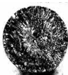
Figure 10. Gas void at the fracture surface of the molybdenum ingot (In the vicinity of a PM fragment, the center).
