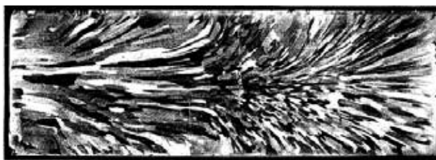
Figure 11. Macrostructure of the molybdenum ingot of 1m length after the EBM run at 0.2 \text{ kg min}^{-1} (left part) and 2.0 \text{ kg min}^{-1} (right part).
