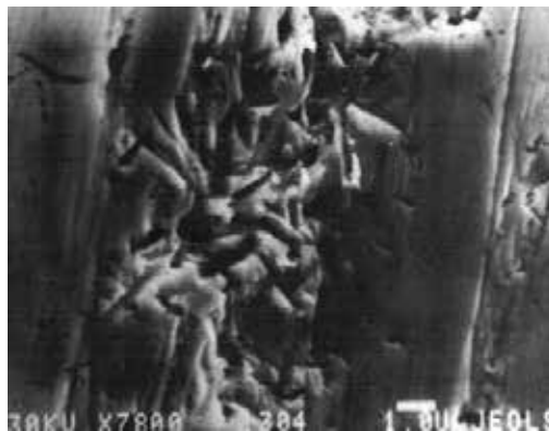
Figure 19. Cracks and pores in hot-rolled sheets of the “low” density tungsten ( \times 7800 ). The plane is perpendicular to the rolling direction.
