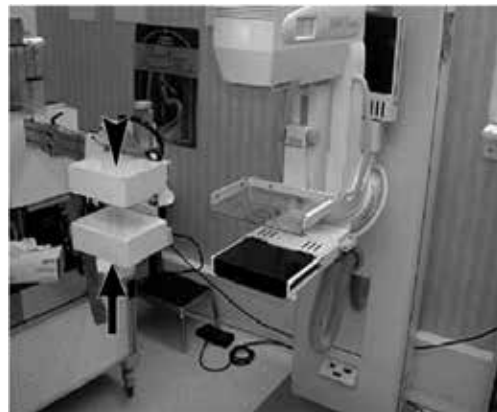
Figure 8. Image of the Duke University - Jefferson Laboratory PEMsystem positioned in a mammography unit. The PEM detectors are highlighted by black arrows. From [34].
