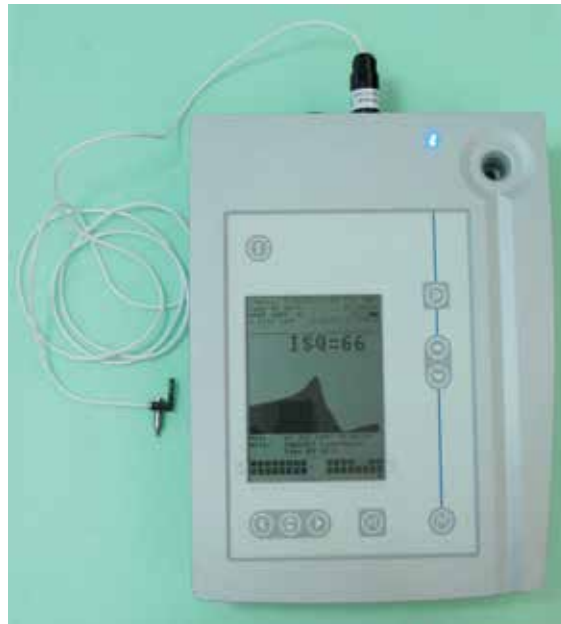
Figure 14. Osstell instrument used to determine implant stability.
