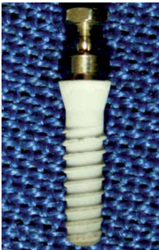
Figure 7. Hydroxyapatite-coated titanium implant.
