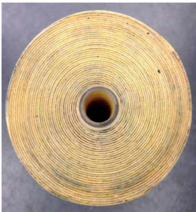
Figure 6. Used RO membrane from a home dialysis WRO machine
