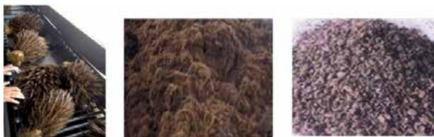
Empty fruit bunch (EFB) Palm mesocarp fiber (PMF) Palm kernel shell (PKS)
