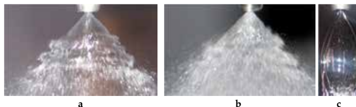
Figure 5. Comparison of the expiration of different liquids at the same mass flow through the cylindrical nozzle without air supply at G_A = 0 , G_F = 5 g/s: (a) water, (b) kerosene, and (c) mixture of diesel with rapeseed oil (50%–50%)
