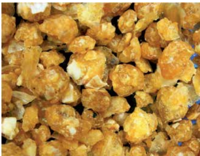
Figure 1. Corn-based Distillers Dried Grains with Solubles (DDGS) is currently the most common coproduct available from U.S. fuel ethanol plants (Photo courtesy of Rosentrater).
