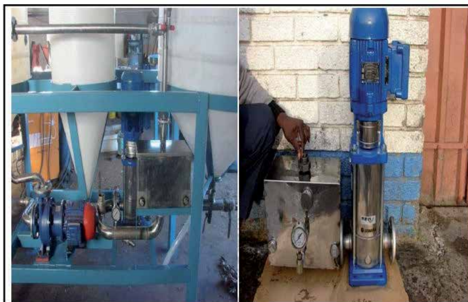
Figure 2. Stirred tank reactors using the jet mixing technology
