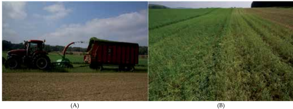
Figure 3. Prototype alfalfa leaf stripper. A. Process of stripping the leaf fraction from alfalfa plants. In this prototype machine, harvesting stems was a separate activity from harvesting of the leaf fraction. The stem fraction was left standing in the field until leaves had been removed and then stems were cut and chopped for ensiling. Next generation harvesters would combine these two operations into a single pass over the field. B. Alfalfa stems with 80-90% of the leaves removed.
