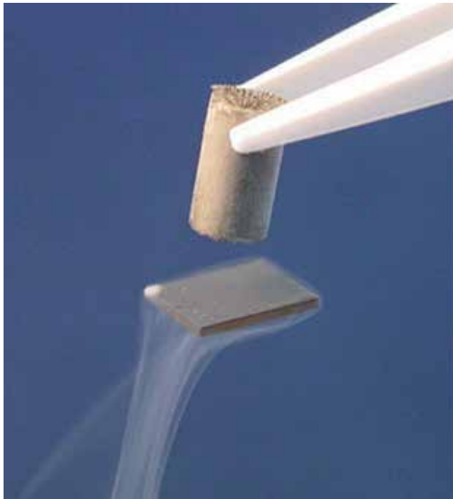
Figure 6. Levitation of 1 \text{ cm}^2 substrate with 100 \text{ nm} YBCO film under \text{SmCo}_5 permanent magnet.
