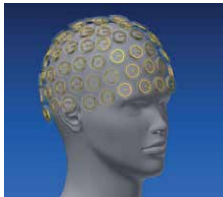
Figure 22. Example of positioning more than 100 encapsulated HTM-D20 magnetometers around a 3D model of the head of an adult human.
