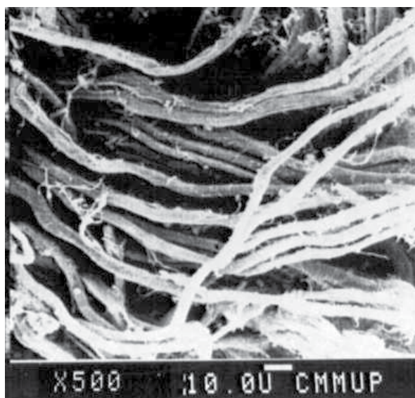
Figure 1. SEM micrograph of internal structure of leather . Adapted with permission from Ref. [14]. Y [1995] American Physical Society.
