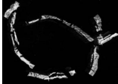
Figure 18. Topogram of angular scanning of a cross-section of W tube crystal.
