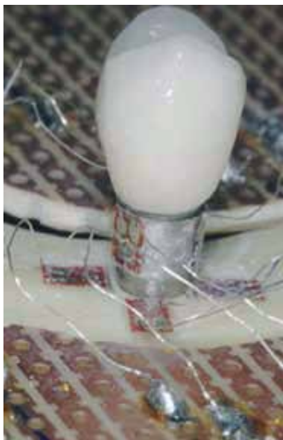
Fig. 8. A bone simulated model was used to quantify the tension around the cervical area of the implant when the restoration is connected.
