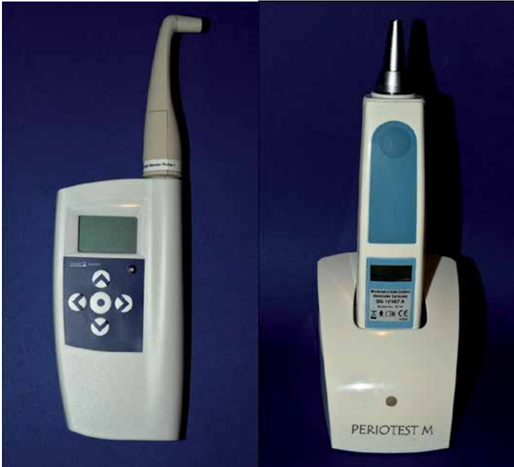
Fig. 20. Osstell mentor (left) and Periotest M (right)
