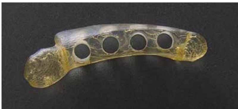
Fig. 6. Fabrication of the guide by stereolithography machine.
