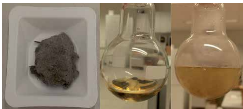
Figure 14. One-step dissolution and hydrolysis of fiber sludge (left) using tailored ionic liquid (middle, tailored IL and fiber sludge) and regeneration of cellulose (right).
