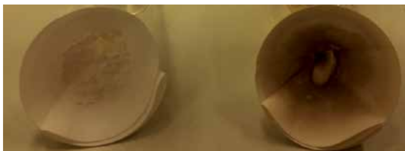
Figure 15. Filtrated regenerated cellulose (dry filter paper) after dissolution of cellulose with (right) and without (left) water in a tailored ionic liquids.
