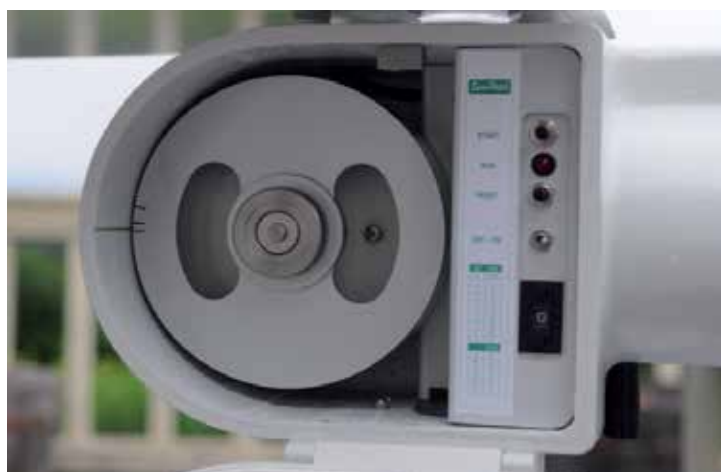
Figure 2. Burkard SporeWatch sampler Cylinder with 7-days or 24-hours periods of selection in Krasnodar
