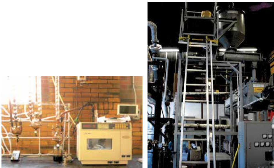
Fig. 1. Batch and continuous microwave assisted pyrolysis (Courtesy: Dr. R. Ruan, University of Minnesota, MN, USA)
