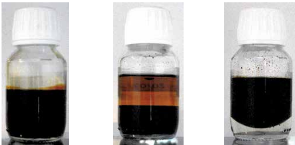
Fig. 5. Pictures of pyrolysis oil (left), mild HDO (middle) and 2 nd stage HDO (right) products
