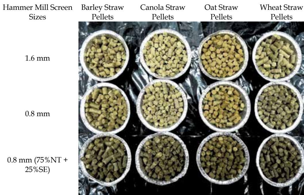
Fig. 4. Photograph of pellets manufactured using a pilot scale pellet mill for non-treated (NT) straw at 1.6 and 0.8 mm hammer mill screen size, and customized grinds at 0.8 mm screen size having 25% steam exploded (SE) straw.
