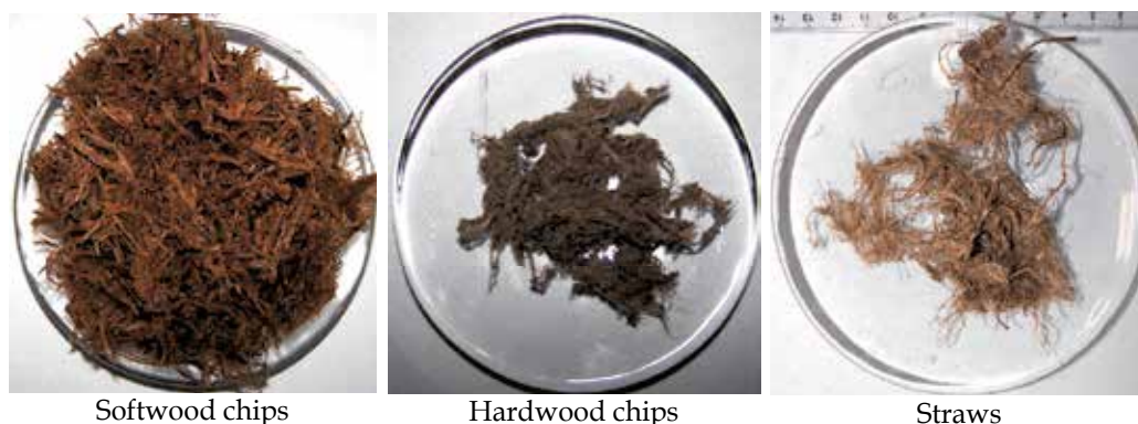
Fig. 2. Lignocellulosic matrix obtained after a non-catalytic steam treatment of different biomasses with a severity factor between 3 and 4
