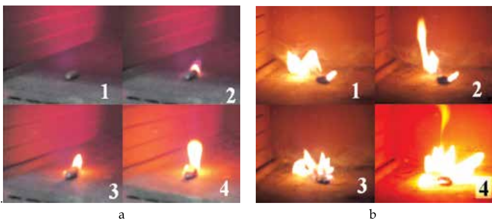
Fig. 5. Process of inflammation: a) wood chip, b) date seed; 1-4 – stages of inflammation from time of placing particle into the muffle (1) separated by 20 s.
