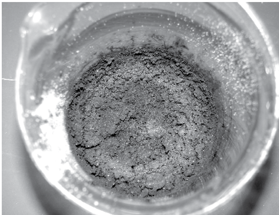
Fig. 17. Mid-value or low-value fractions from DDGS (such as fiber) can be thermochemically converted into biochar, which can subsequently be used to produce energy, fertilizer, or as a precursor to other bio-based materials.
