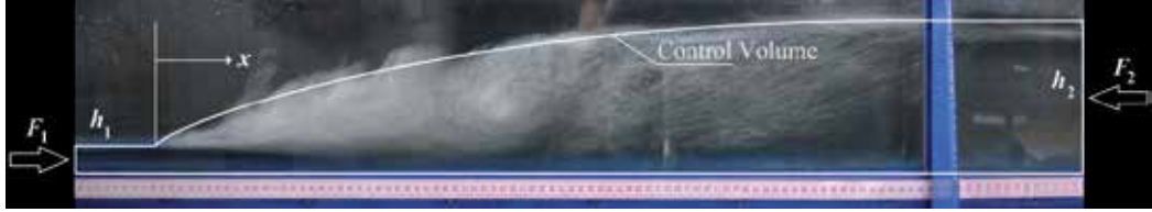
Figure 2. Hydraulic jump and adopted control volume. The photograph was taken to show the air bubbles ascending, and the outlet section located where no air bubbles are present.
