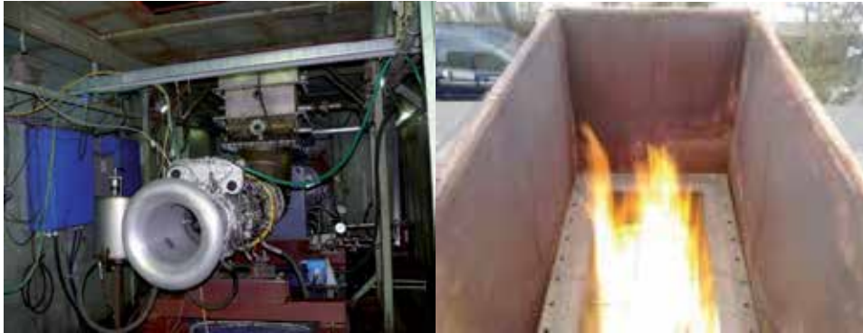
Figure 3. TA2 gas turbine engine mounted on the stand (left) and afterburning installation (right)
