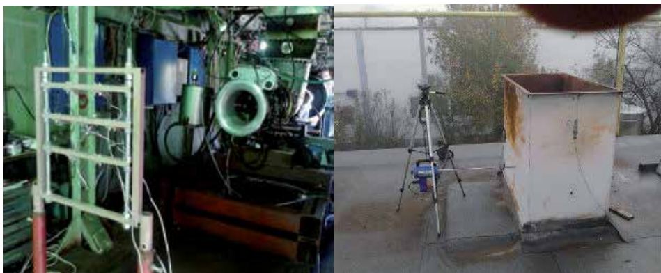
Figure 18. Experiments regarding the injection of water in TA2 gas turbine (left) and gas analyser PG 250 (right)
