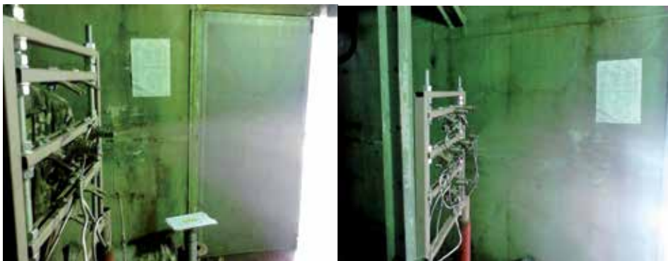
Figure 17. Water spraying tests, using a liquid fuel atomizer from TV2-117A gas turbine
