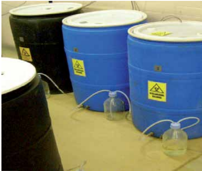
Figure 20. Disintegration barrels used to assess plastic fragmentation in an aerobic composting environment according to AS ISO
