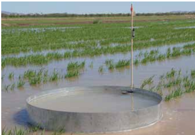
Figure 5. Class A Evaporation Pan with a stilling well located near one edge (also shown is a Baro-Diver to measure variations in atmospheric pressure).
