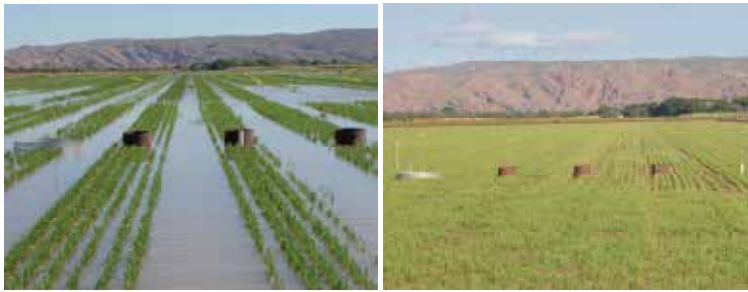
Figure 3. Field setup of lysimeters and Class A Evaporation Pan for two planting configurations.
