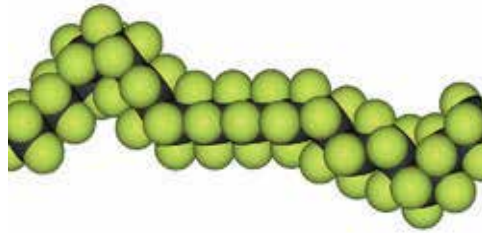
Figure 1. Typical interwinded PTFE polymer. Due to strong intermolecular forces, the polymer chains are tangled. Due to its chemical inertness, PTFE cannot be cross-linked.
