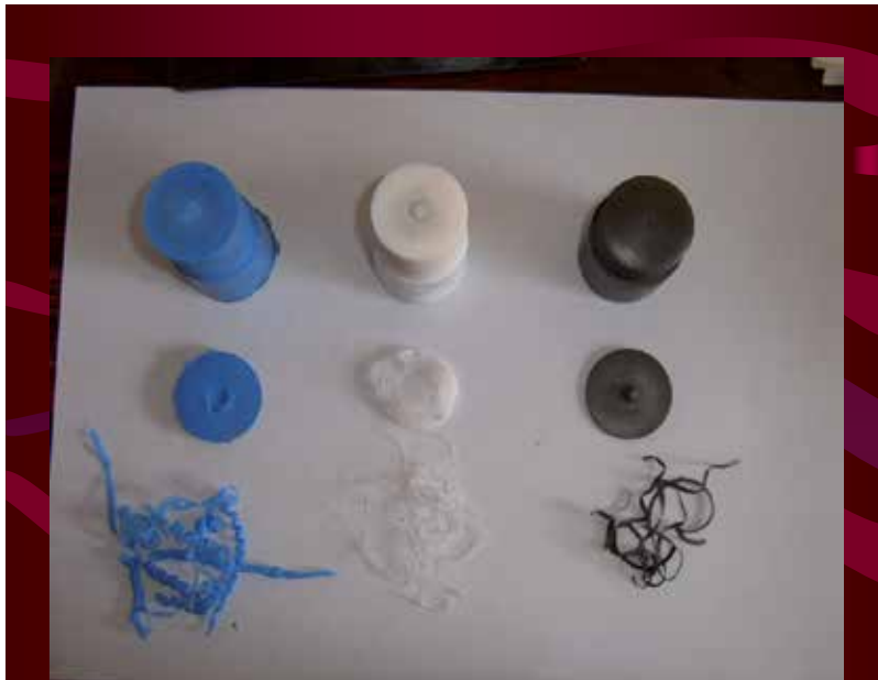
Figure 5. Sintered rods made from blue pigmented PTFE, glass mixed PTFE and carbon mixed PTFE
