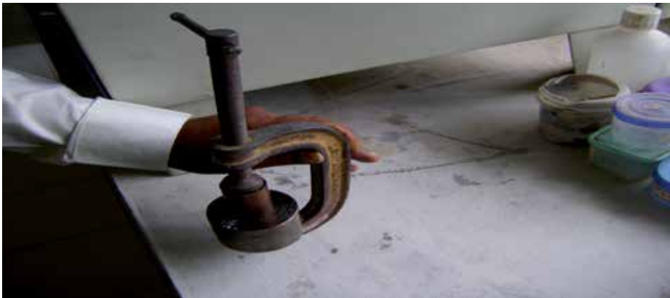
Figure 22. Cold pressed pellet along with the die and plunger being pressurized with the help of a C-clamp
