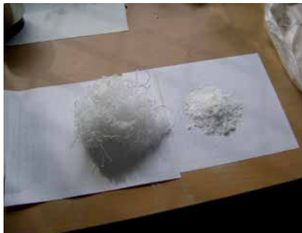
Figure 6. PTFE scrap before (left) and after gamma irradiation (right)
