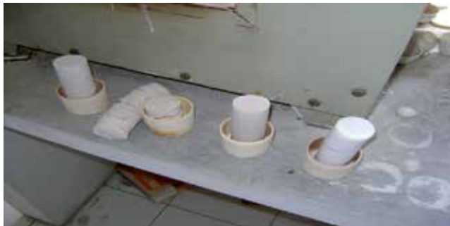
Figure 20. Sintered rods at atmospheric pressure – note pellets from 100% virgin scrap (second from left) crack and pop out perhaps due to the release of volatile gases whereas the pellet from 100% virgin PTFE (extreme right) are milky white in color and exhibit good integrity on sintering at atmospheric pressure.
