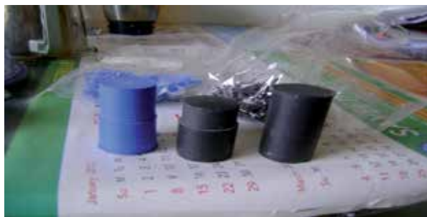
Figure 18. Fillers like graphite or pigments normally do not melt or agglomerate nor interact with PTFE during sintering at atmospheric pressure but this is not the case with reprocessed PTFE when used alone or used as a filler with virgin PTFE
