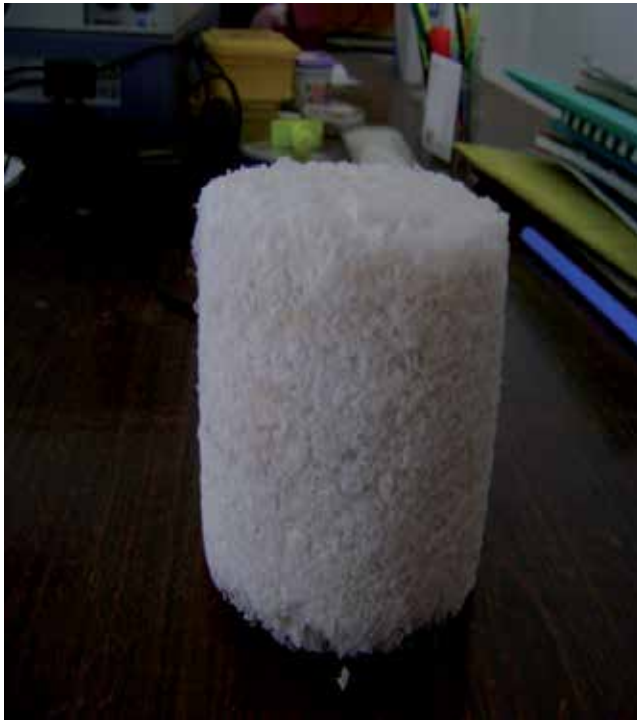
Figure 13. Shredded PTFE scrap after pre-heating treatment
