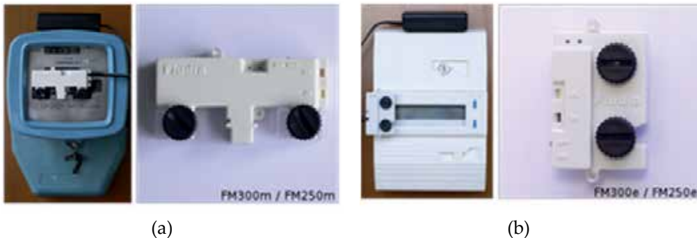
Figure 8. Flundiometer: (a) monitoring module for electromechanical power meters (b) monitoring module for electronic power meters [40].
