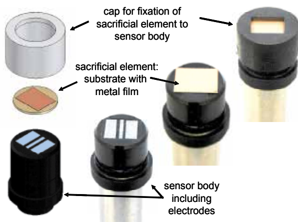
Fig. 2. Setup of the sensor for evaluation in the laboratory
