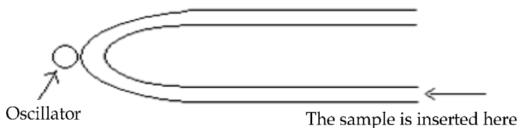
Fig. 7. U-shaped tube of digital density meter.
