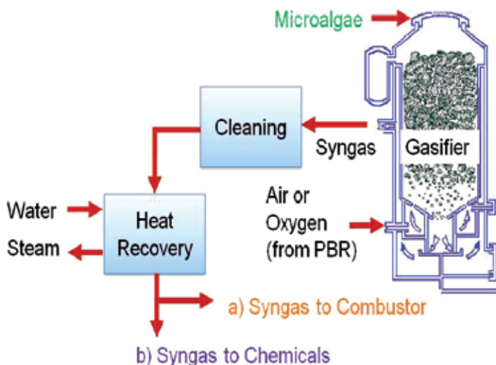
Fig. 5. Integrated microalgae production and gasification
