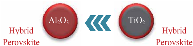
Figure 17. Switching \text{TiO}_2 to an \text{Al}_2\text{O}_3 in Gratzel perovskites solar cell
