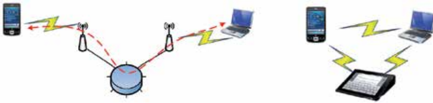
Figure 1. Infrastructure based networks (left) and Ad hoc networks (right)
