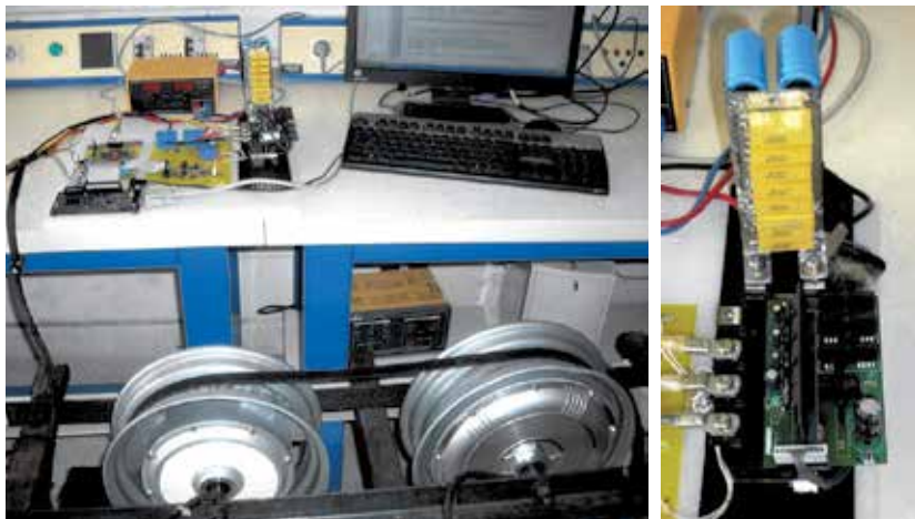
Fig. 8. Experimental setup for the in-wheel brushless motor drive validation and the IPM based power circuit.
