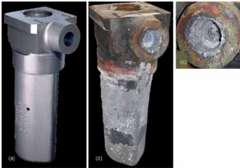
Figure 16. Goosenecks of hot chamber die casting machine: (a) part before exposure to liquid magnesium; (b, c) gooseneck after service with extensive corrosive attack [85].
