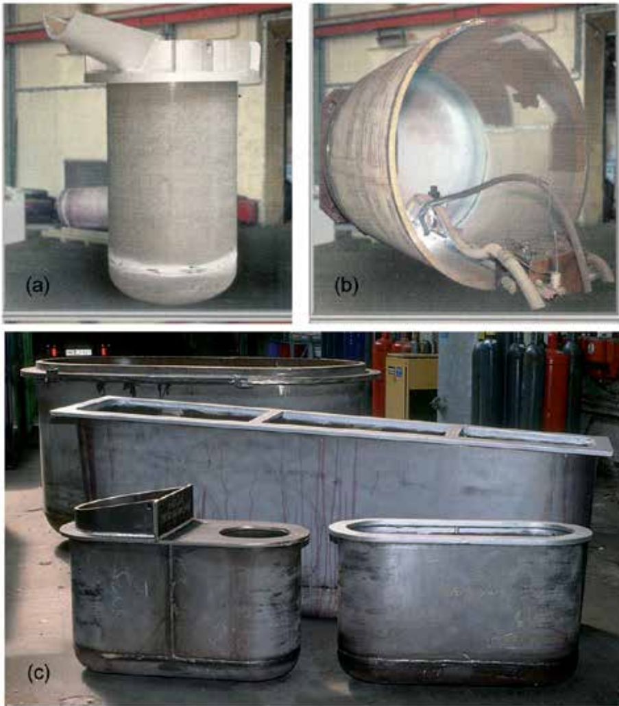
Figure 9. Commercial processes requiring equipment resistant to liquid magnesium: (a, b, c) crucibles for magnesium melting [83];
