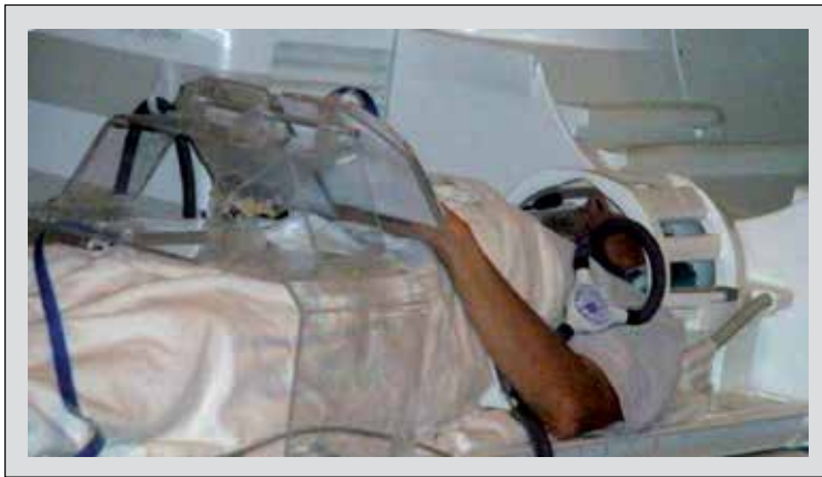
Figure 5. A subject on the scanner bed operating our novel multimodal MRI-compatible drawing device. The plexiglass gantry supports a drawing tablet while a fiber-optic drawing stylus captures and records the drawing movements with high precision. The motion capture information synchronized with the fMRI allows the effect of behavioral events to be analyzed to high precision.
