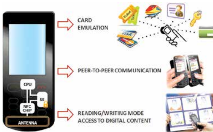
Fig. 1. NFC communication modes
