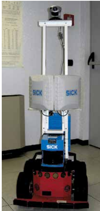
Fig. 1. The mobile robot Pioneer P3AT equipped with two RFID antennas and a laser range scanner.
