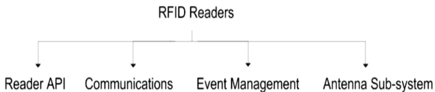
Fig. 11. RFID reader logical components
