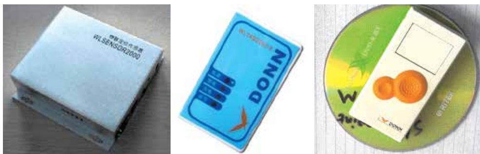
Fig. 10. The indoor positioning sensor and active RFID positioning tag
