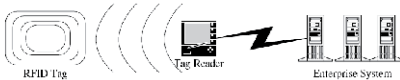
Fig. 3. A typical RFID system (Roberts, 2005)
