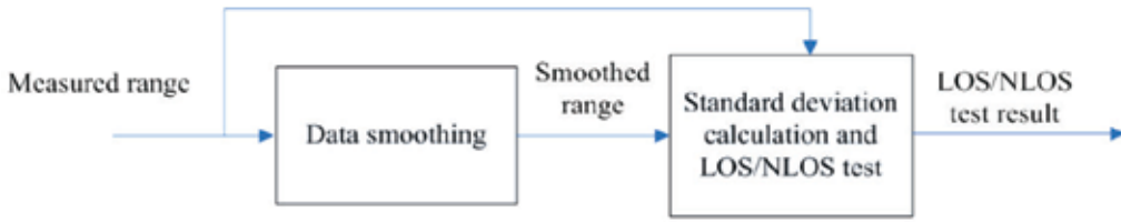
Fig. 2. Identification of LOS/NLOS propagation status
