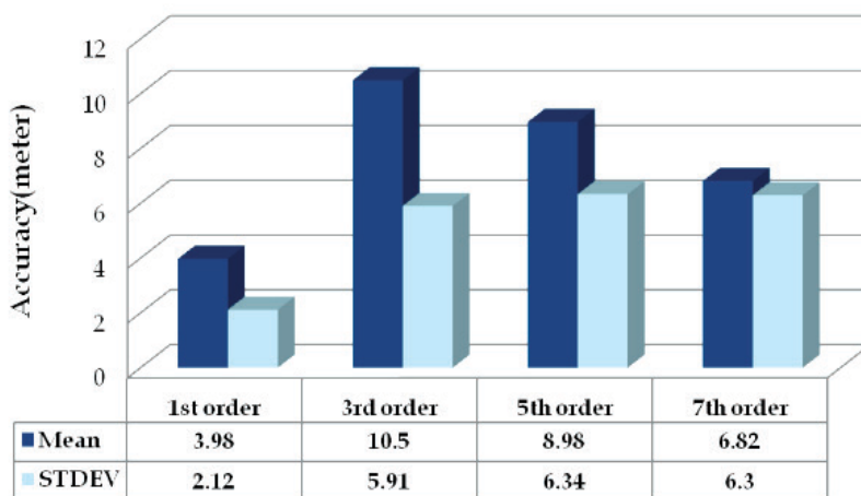
Fig. 11. Statistics of the positioning error based on the curve fitting models.
