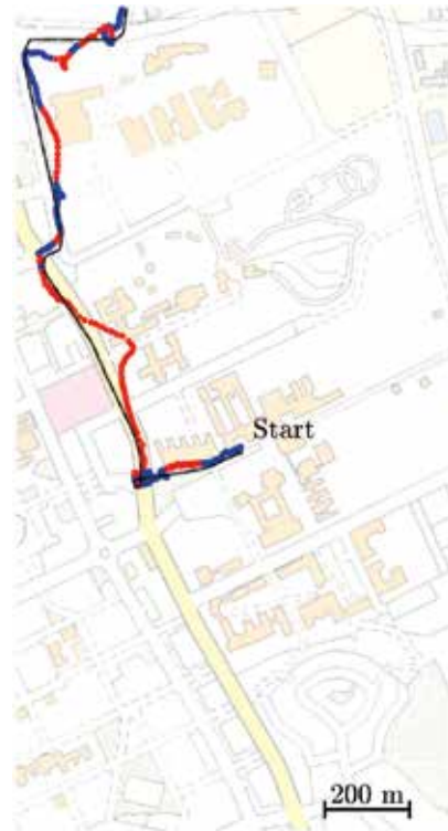
Fig. 3. An example of REKF using real GPS-measurements
