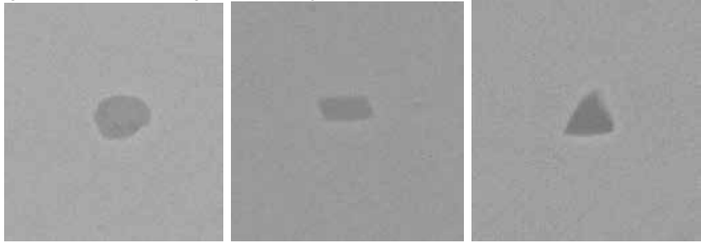
Fig. 69. Shape of inclusions in a stainless steel
