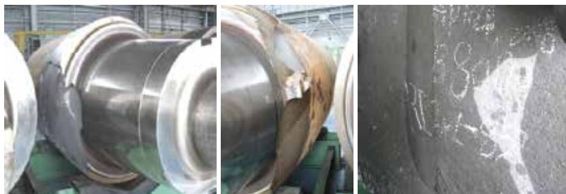
Fig. 2. Spalling of backup rolls in roughing mill of 2250HSM
