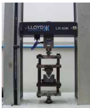
(b) V-bending die set assembled on tensile test machine
