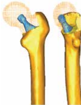
Fig. 6. Meshing of proximal fémur with stem
