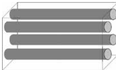
Fig. 4. 3D model of a oriented long fibre composite
