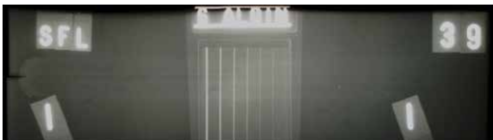
Fig. 16. X-ray image of specimens produced on AA2024-T4 with void defects Type III
