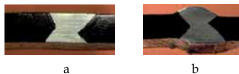
Fig. 16. Toe finish, a) toe emery eliminated, b) bulge emery smoothing.
