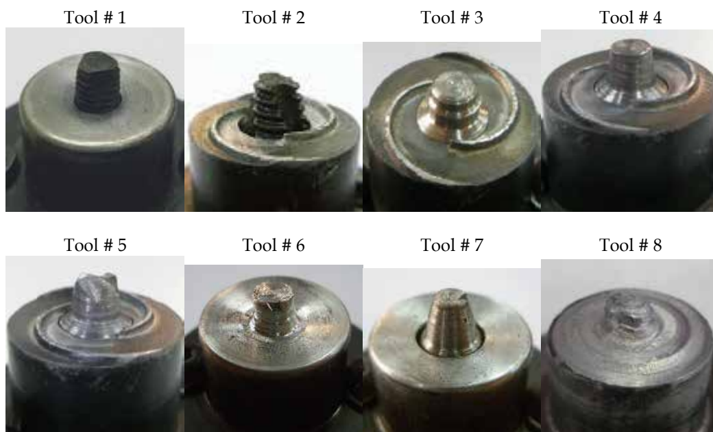
Fig. 9. FSW tools used to produce defect and non defect condition on AA2024-T4 and AA5083-H111
