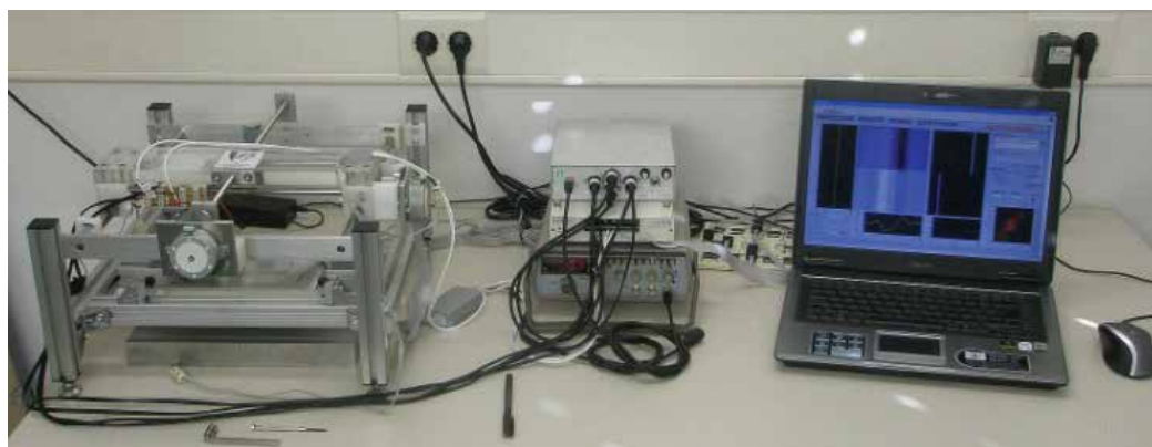
Fig. 25. NDT system overview: laboratory apparatus for inspecting FS welds: the mechanical support system device and the computational data acquisition device.
