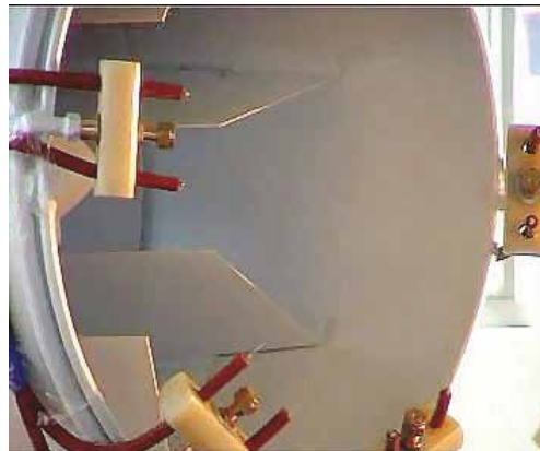
Fig. 4. Fixing of electrodes for sprayer
