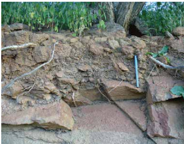
Fig. 2. Windhoek soil profile measuring 20 cm from the Northern Industrial area. The bottom of the pen shows the bedrock-soil profile contact. Note the immaturity of the soil horizon.
