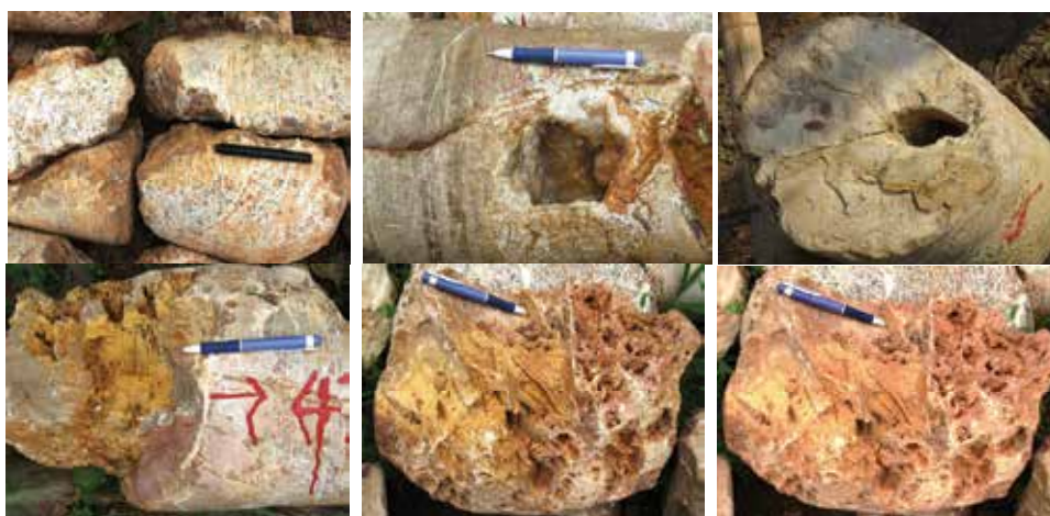
Fig. 5. Corrosion of rock core samples
