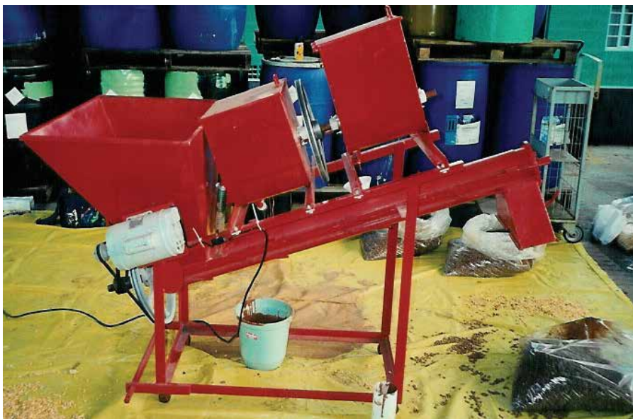
Fig. 18. Seed treatment machine, used to test the application of camouflage in corn seeds. On the floor, in plastic sacks, results of three tests of camouflage by varying the amount of carbofuran syrup, dye powder and water.
