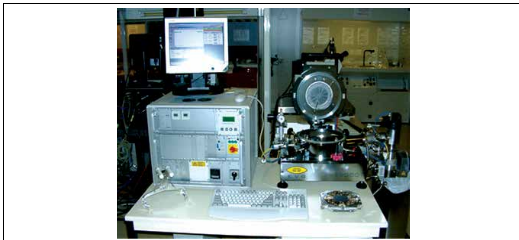
Fig. 6. Wafer bonding: EVG bonding machine used for wafer pre-bonding (the bonding is finished using a classical press)
