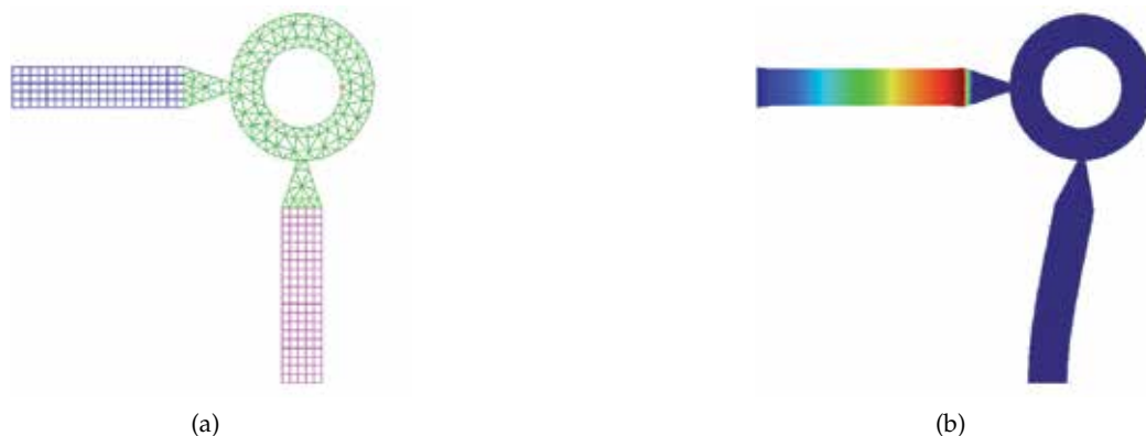
Fig. 16. Piezoelectric revolving drive: (a) FE grid; (b) Strongly scaled (factor of about 150) mechanical deformation for a characteristic time step, when the left actuator is at maximal load.
