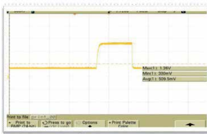
Fig. 13. Voltage across PV panel
