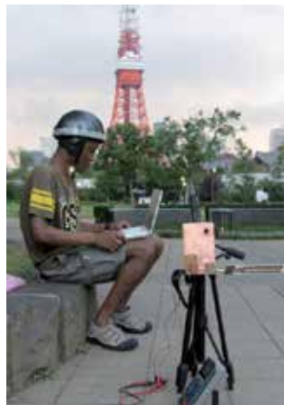
Fig. 15. DTV energy harvesting in a park at some line of sight from the base station.
