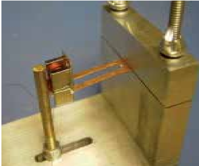
Fig. 20. Generator A-showing four magnets attached to a copper beam and wire-wound coil.
