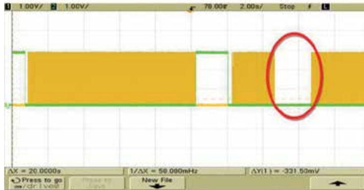
Fig. 16. No switching at Gate of NMOS3 when V_{ref} is less than V_{pv}
