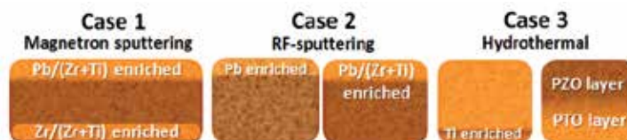
Fig. 7. Common compositional profiles for PZT thin film fabricated by sputtering and hydrothermal techniques. Case 1: based on the work of Vidyarthi et al., 2007; Case 2: Chang and He, 2005; Suchanek et al., 2002; Case 3: Morita et al., 1997; Ohba et al., 1994.
