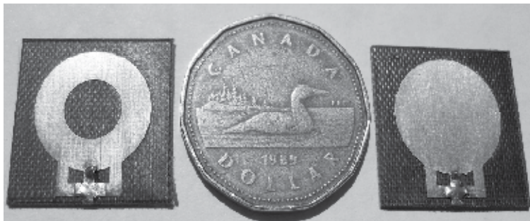
Fig. 18. Circular monopole antennas of Fig. 3a and Fig. 3c etched each on a 22x22mm 2 substrate with \epsilon_r=2.5 , height=0.8mm. Antennas are compared to the Canadian Dollar Coin before being mounted on the Aluminium ground plane
