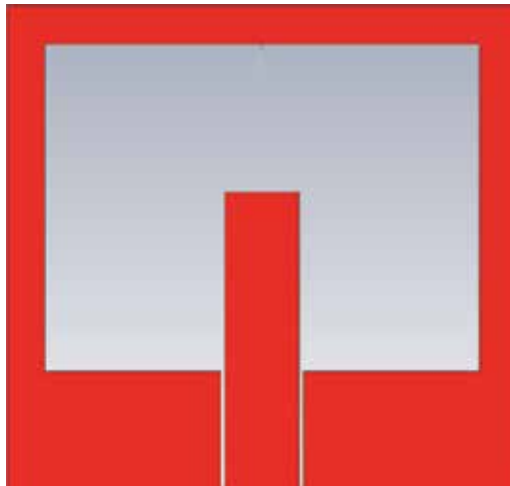
Fig. 1. CPWG topology comprises both electric-source and magnetic-source.
