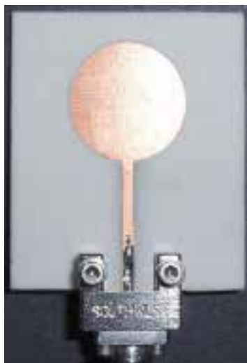
Fig. 1. The prototype of the proposed simple fed CDM antenna
