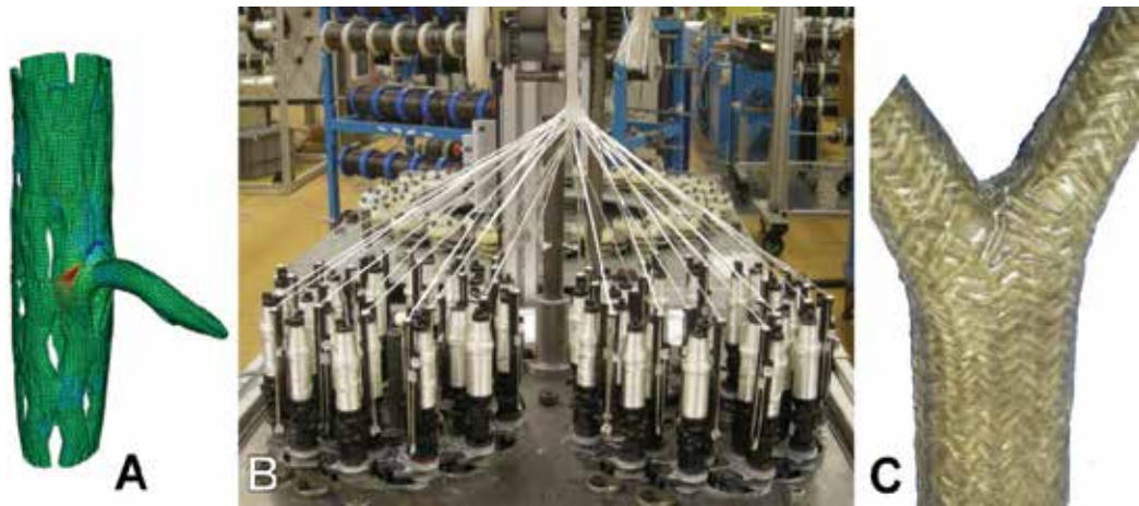
Fig. 28. (A) Simulated notch stresses in a stem-branch attachment region of a columnar cactus, (B) double braiding unit for producing branched braidings and (C) prototype of a braided Y-shaped preform. © (A) ILK Dresden, (B, C) ITV Denckendorf.
