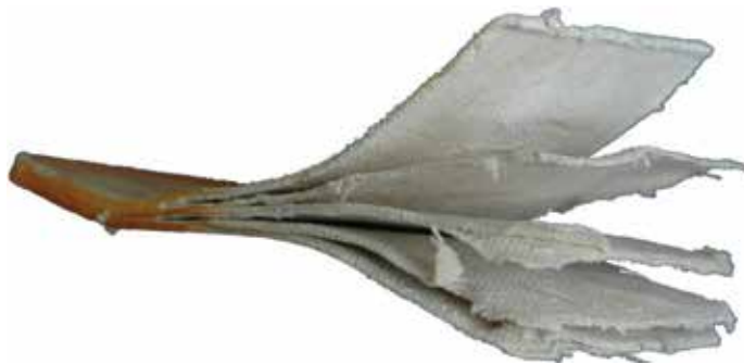
Fig. 15. Delaminated technical composite structure © PBGF.
