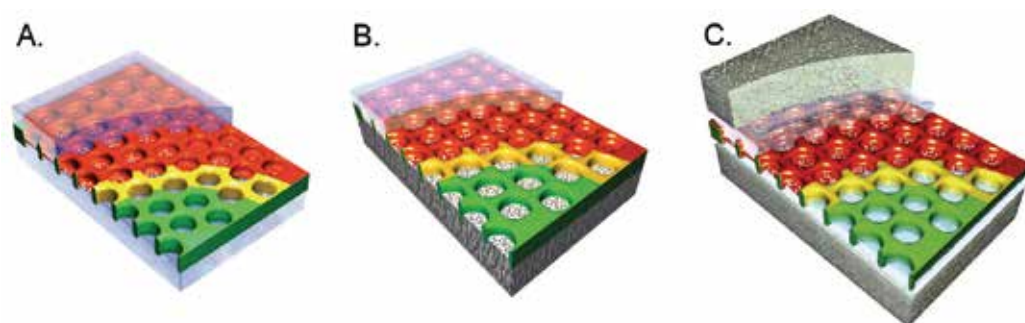
Fig. 1. Biomimetic membrane array designs using micro-structured ethylene tetrafluoroethylene (ETFE) as scaffold. A) ETFE membrane scaffold for freely suspended planar membrane arrays. B) Composite half-sandwich membrane scaffold consisting of an ETFE partition partly embedded in a porous support structure to create individually well-defined wells (grey). C) Complete composite scaffold sandwich structure. Shown in the illustrations are the ETFE membrane scaffold (green), surface modifications of the ETFE scaffold (yellow), biomimetic membranes (red), proteins (white), aqueous layers or hydrogel polymers (transparent) and porous supportive structures (grey).
