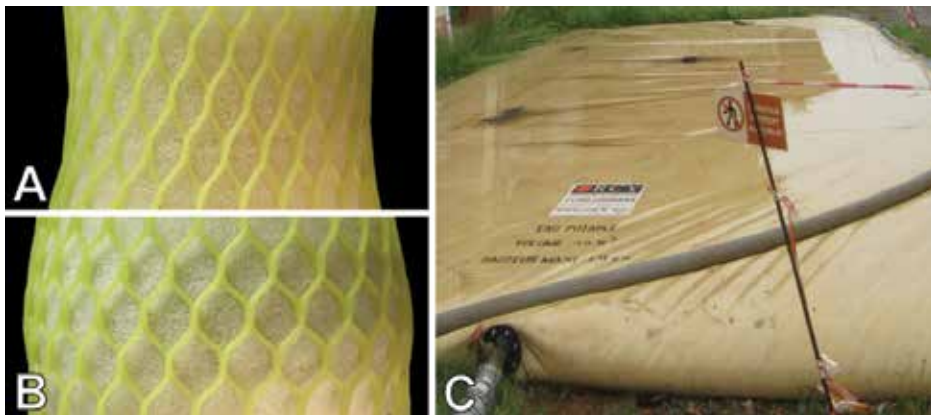
Fig. 23. Potential technical implementation for flexible hull structures. (A, B) Demonstrators combining a cellular matrix consisting of closed-cell foams and inextensible fibers, (A) undeformed state, (B) deformed state, (C) conventional flexible tank as an example for a potential technical application. © PBGF.
