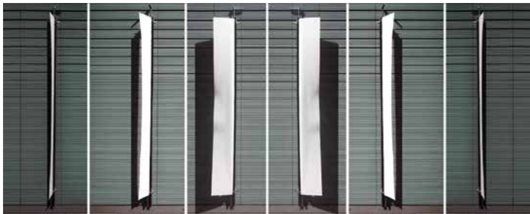
Fig. 12. Demonstrator for a façade shading system able to bend sideways up to an angle of 90° inspired by the kinetic system found in the flower of Strelitzia reginae . Torsional buckling and displacement of the lamina are induced by slightly bending the supporting rod. © itke University of Stuttgart.
