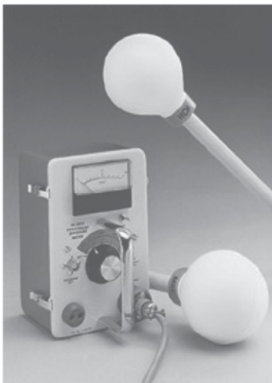
Fig. 8. Electric and Magnetic Field meter. Readout device is same for E and M probes
