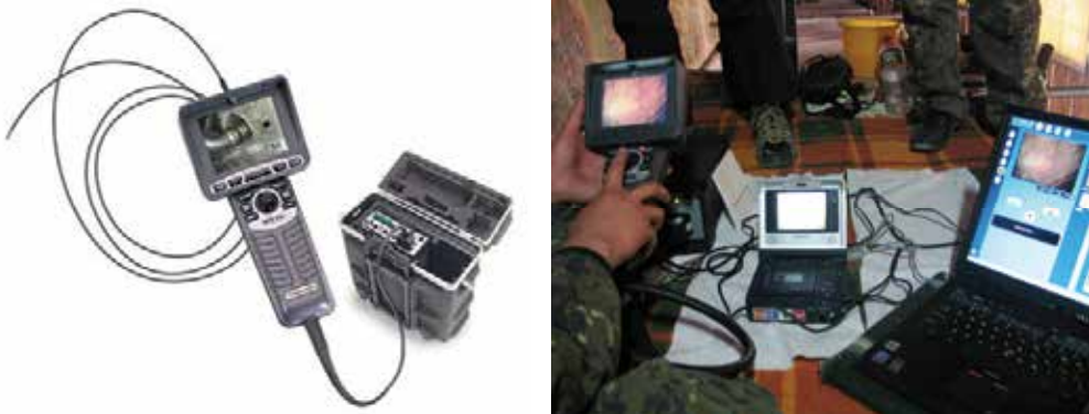
Fig. 15. XL PRO Video probe made by EverestVIT for remote visual test
