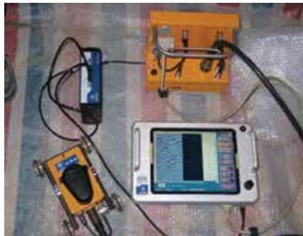
Fig. 4. RAMAC/GPR made by MALÅ GeoScience
