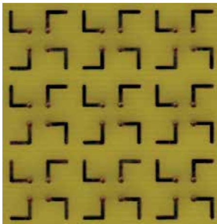
Fig. 6. Photograph of a structure similar to the shown in Fig. 3, but manufactured by means of Printed Circuit technology.
