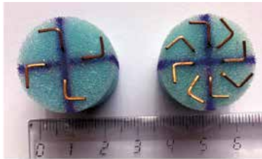
Fig. 18. Cylindrical samples used for the experimental determination of chiral effect by using a waveguide setup.
