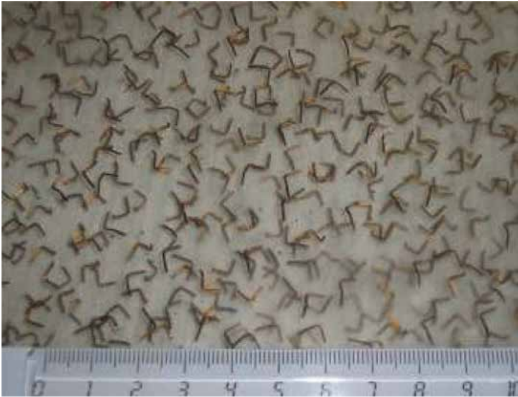
Fig. 2. Crank-based artificial chiral material. Chiral elements were produced from a 0.4 mm diameter and 12.6 mm length copper wire by bending in three segments by two 90 angles, all with the same handedness. The elements were dispersed in an epoxy resin with a low curing temperature (Molina-Cuberos et al., 2009).
