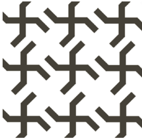
Fig. 4. Planar chiral structure made by arrays of gammadions arranged in two-dimensional square gratings (Papakostas et al., 2003).
