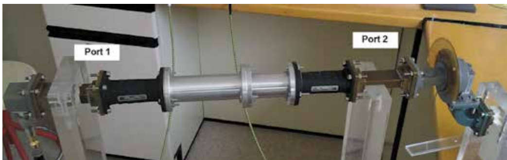
Fig. 8. Waveguide setup for the experimental determination of the rotation angle produced by a chiral material in X-band. A cylindrical sample is located in the circular waveguide and fed through port 1. The transmitted wave is measured in port 2 by a rotating connection, which allows determining the component of the electrical field parallel to the TE_{10} mode of the rectangular wave.
