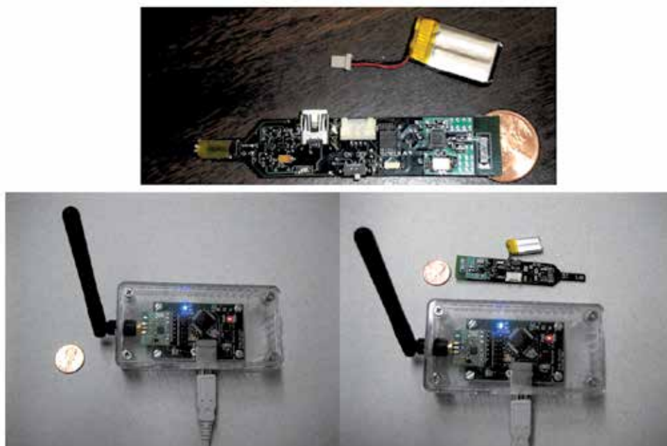
Fig. 34. Photographs of integrated pH sensor (top) and receiver/transmitter pair (bottom).
