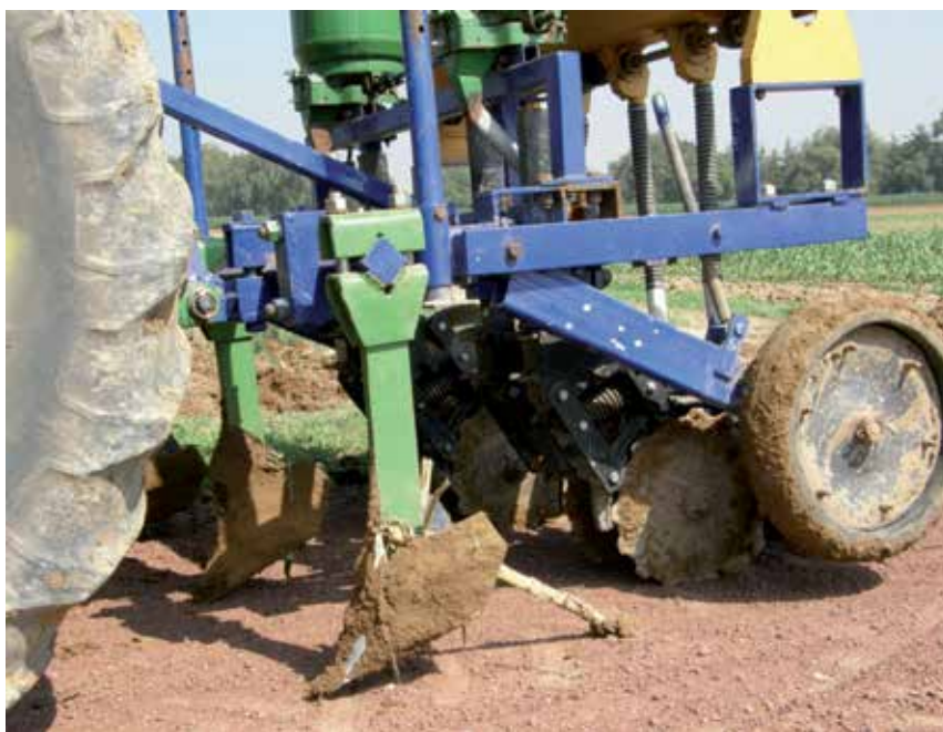
Fig. 5. Prototype of disk-type planter for small-grain cereals and maize developed for the planting system on permanent beds.
