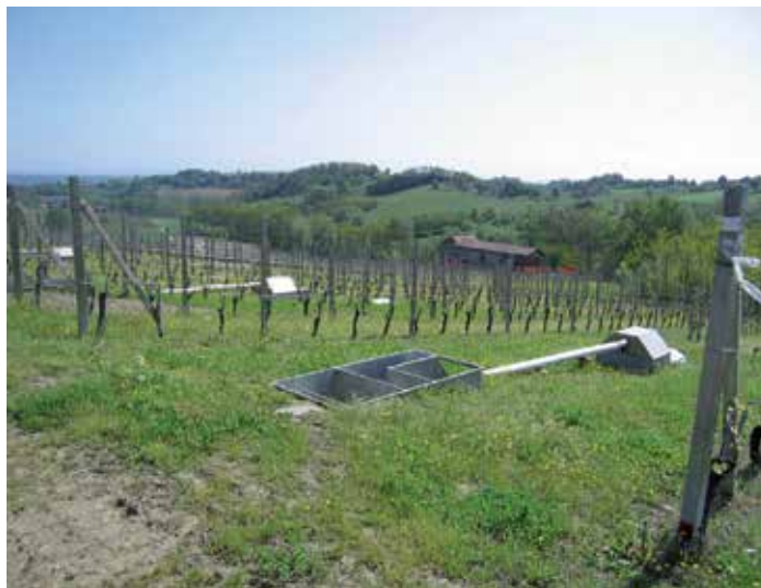
Fig. 7. Sedimentation trap and tipping-bucket device for runoff discharge measurements.
